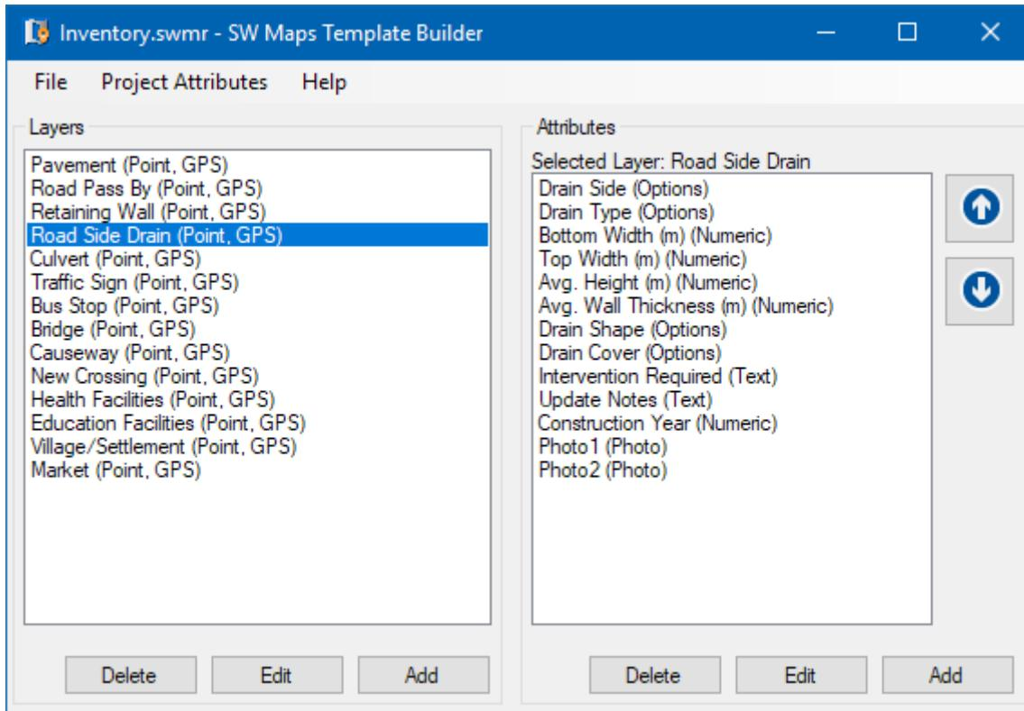
The template builder can be used to create normal (swmt) or read-only (swmr) templates. Read-only templates do not allow the user to add or remove layers and attributes, which makes it suitable for large scale data collection and processing.
