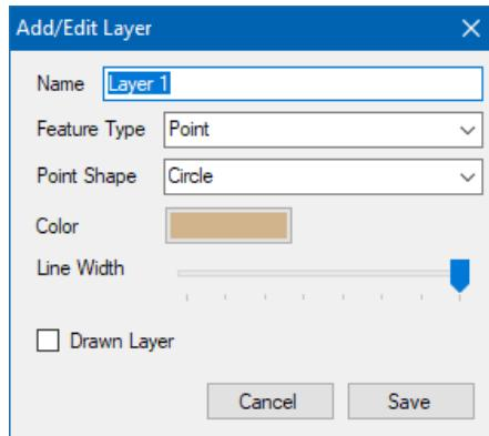
Enter the layer name, select the feature type and define the layer style (point color, line width and point shape)
